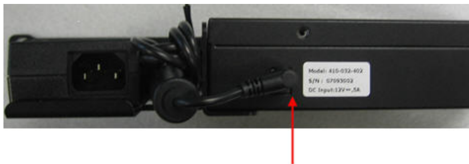
Figure 17 Insert the power supply cable into the connector on the rear panel
